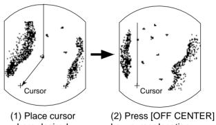
(1) Place cursor (2) Press [OFF CENTER] where desired. key; cursor location becomes screen center. Figure 2-16 Off centering the display
